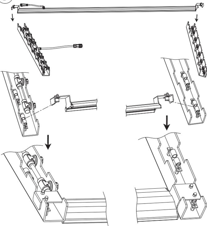
Place the two frames parallel to each other with a distance of 41 inches (105cm) on a flat table, and click each light bar into the frames one by one.
