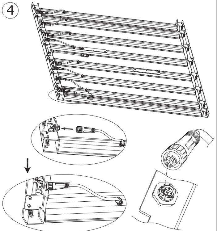
Insert the male connectors (connected to the light bars) into the female connectors (mounted on the frames), and securely fasten the locking rings by rotating them tightly.
